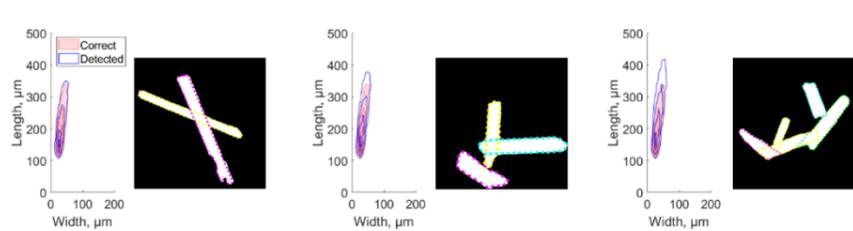
In the final evaluation, the sizes of the original particles were compared to those of the detected particles, one to one. Defining that a 10% relative error is acceptable, then at the highest overlap intensity tested, the length of 75% and width of 80% of the particles are correctly characterized.
